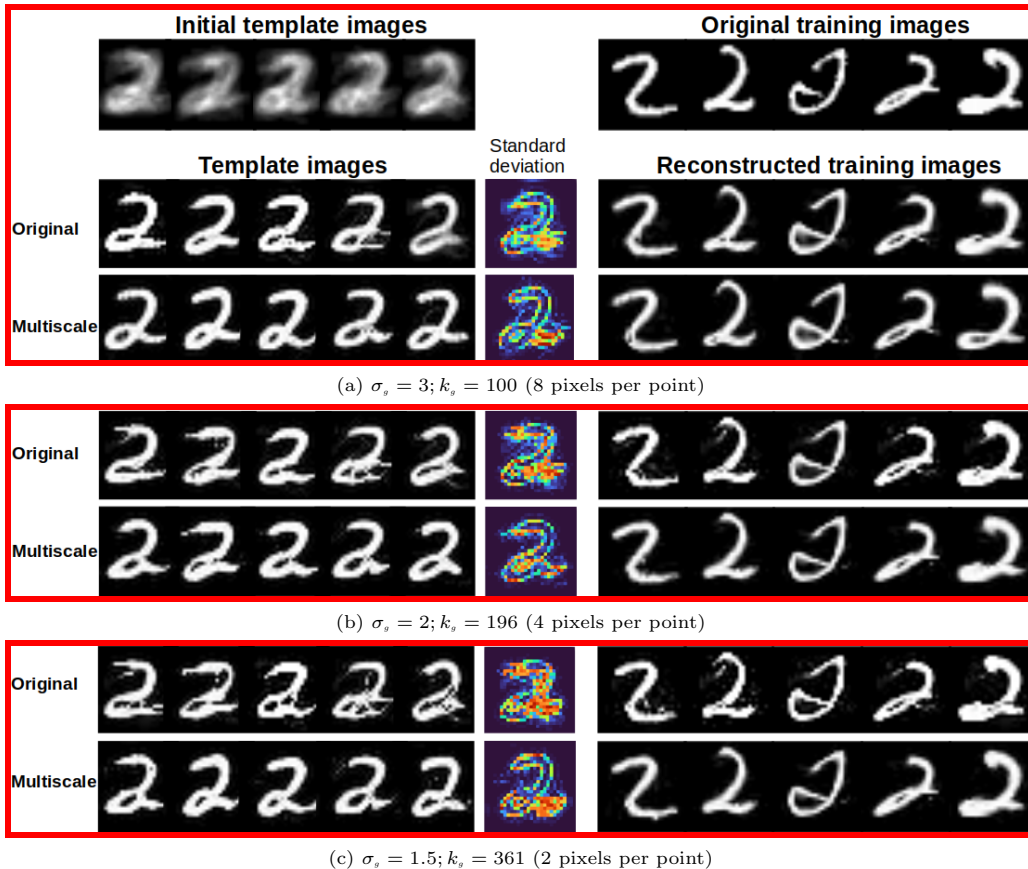
Fig. 9 Estimation of the template image by the original LDDMM and the LDDMM combined with multiscale optimization on the dataset of handwritten digits with different values of \sigma_g . For each experiment, five template images (estimated with non-intersecting training sets) and their standard deviation image are presented on the left, along with the template image from the first training set warped to the first five training images on the right. \sigma_g : width of the Gaussian kernel; k_g : corresponding number of control points.
